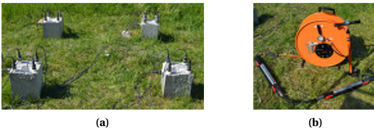
Figure 4.6: Measurement setup for the tests on the free-top piles (a) instrumented with six accelerometers at each pile head (4 vertical and 2 horizontal) and (b) the down-hole equipment used for measurements at depth within the piles.
